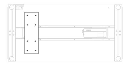
**Step 2:** Place spacers under the track to lift it above any obstacles on the table. Align the spacer holes with the track's mounting holes. Use the 1" spacer alone or combine it with the ¼" and/or ¾" spacers to achieve the desired height.
