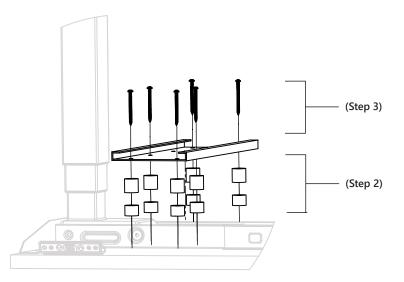
**Step 3:** Using a drill, drive the appropriately selected screw through the track and spacers into the desktop.
