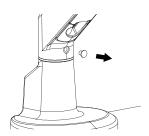
3. Insert and tighten the lock-out screw to make it 180 degree lock-out.
