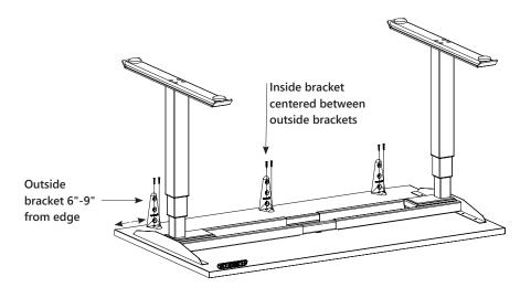
**Step 3:** Place acoustic panel on underside of table surface. Center modesty panel left to right, and attach acoustic panel to L brackets using #8 X ½" Flathead Wood Screws (3).
